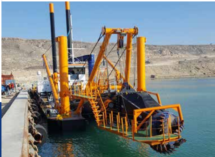
Cutter suction dredger Mangystau with its innovative lightweight platform
