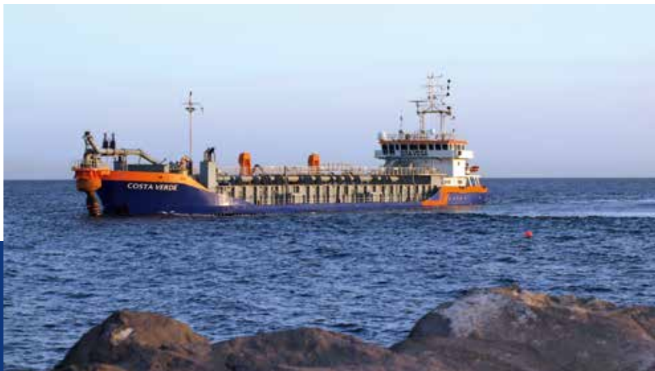
Trailing suction hopper dredger Costa Verde in the Mediterranean
