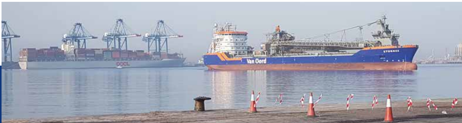
Flexible fallpipe vessel Stornes in Egypt carrying out rock installation work in the West Nile Delta gas field
