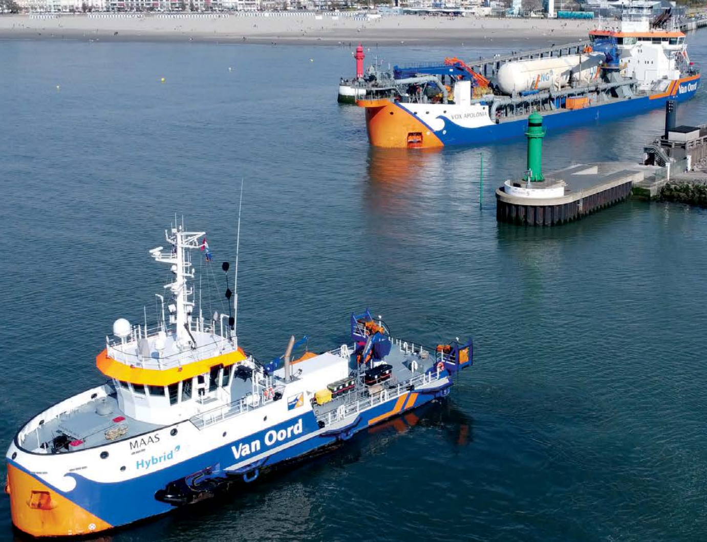
Trailing suction hopper dredger Vox Apolonia and water injection dredger Maas working together on a maintenance dredging campaign in Calais and Boulogne-sur-mer, France.
