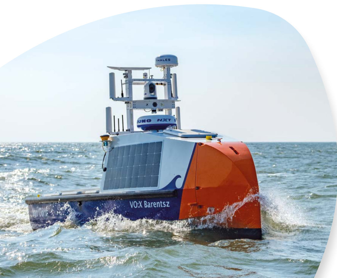
VO:X Barentsz is Van Oord's 5 th unmanned autonomous survey vessel and the first one specialised for operations at sea.
